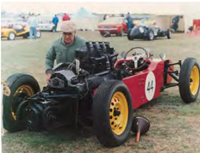
Above: In recent years Warner Mauger has refitted his Stanton Special with a supercharger. Final drive is by chain, two sprockets giving two speeds, to the solid rear axle.
