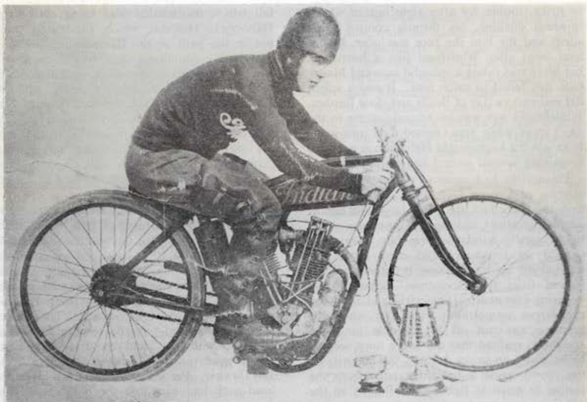
FORMIDABLE COMBINATION. —Percy Coleman and Indian 8-valve, 1918. Note rigid forks and small section high-pressure tyres. Engine featured four vertical overhead valves per cylinder plus auxiliary exhaust ports. Top speed approximately 100 m.p.h.
