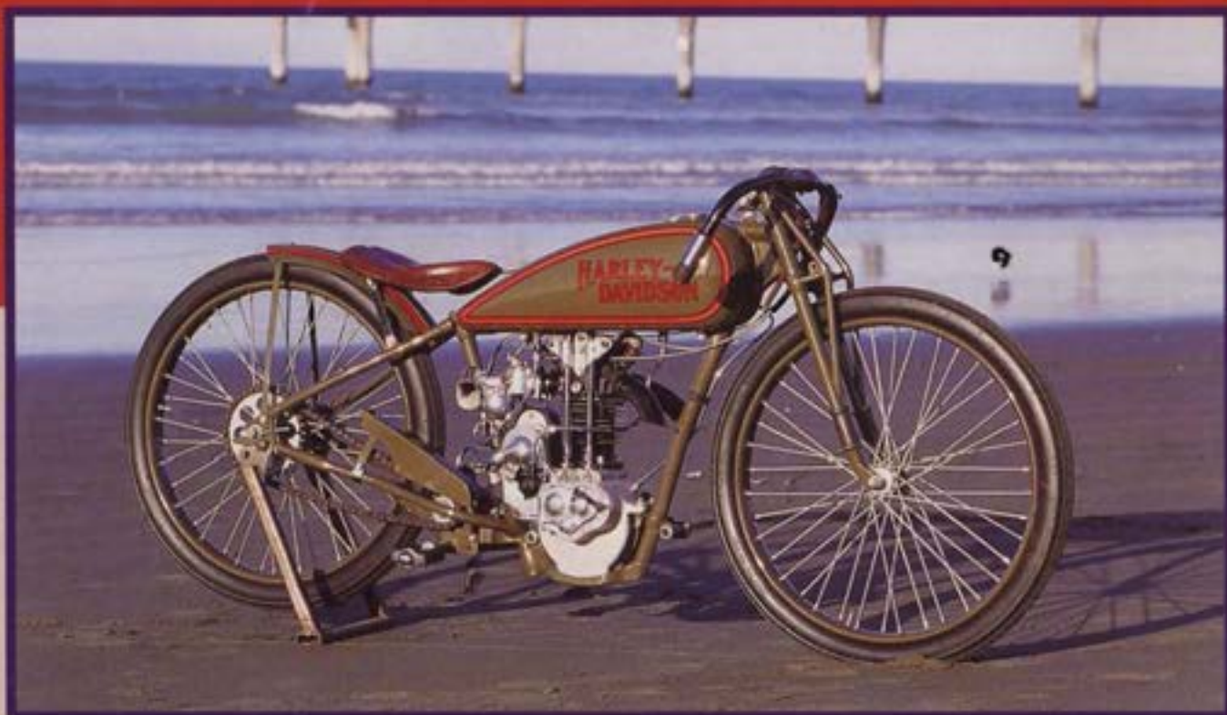
1929 Harley Davidson Peashooter Racer on Firestone 28 x 2 1/4 Racing BE tyres. Owner Joe Grose, photographed by Euan Cameron
