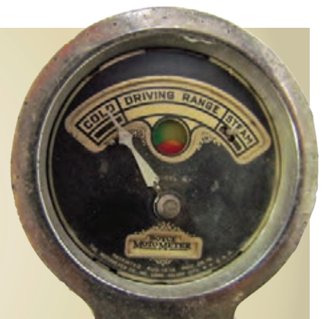
The aperture shows green until overheating causes the pointer to contact the steam pin and bring up a red warning disc. To enable pin resetting no glass was fitted.
