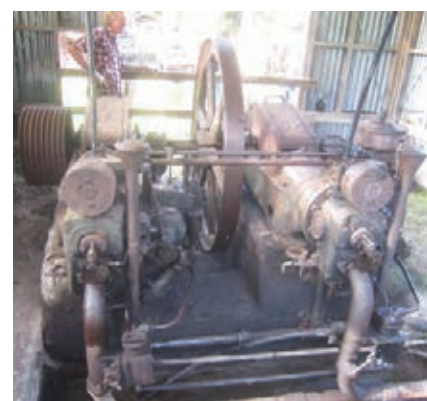
Far North: 1926 Crossley horizontal twin diesel.
