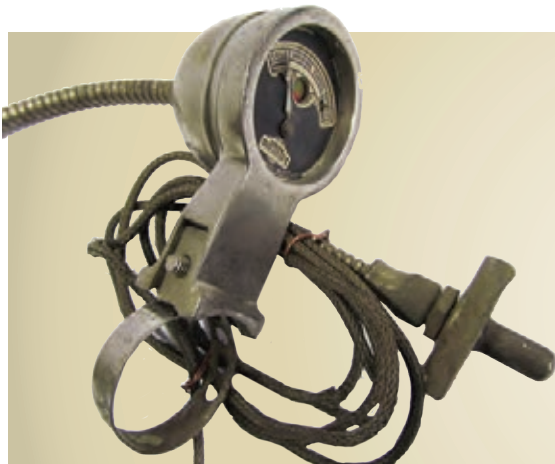
Red Ball distance reading gauge is a quality product, also later available with Chevrolet and Ford Model A logos. They were still being advertised for Ford as late as 1935.
