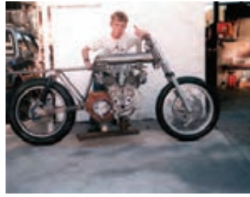
Plywood buck as the design process for gearbox attachment moves ahead.
