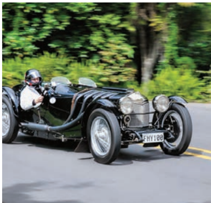
Robert McNair's Riley special betrays its non-Riley motive power by the exhaust pipes emerging from a place Percy never envisaged. The smooth torque from more than 6 litres of DH Gipsy Major propelled the combination to 29.92 seconds, fastest of the day. (Ralph Starck)
