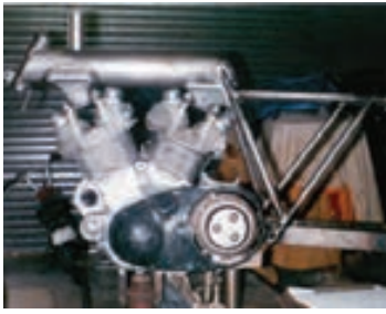
First attempts at matching engine to the frame and testing for gearbox fit.
