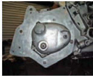
Seating the gearbox in its new mounting plate.
