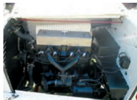
The engine showing the Tillotson carb and original finned aluminium rocker cover
