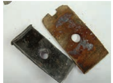
Spot the caster wedge that is now a tool! Spring centre bolt fits through the wedge for positive location.
