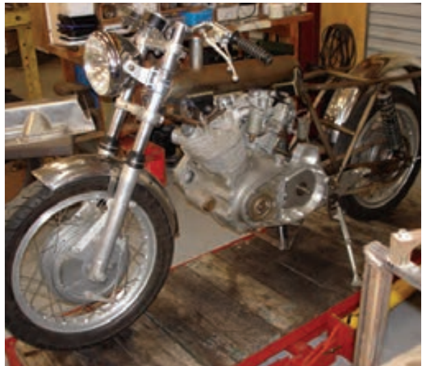
Chain case halves reunited to crank case and swing arm.
