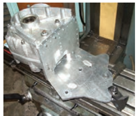
Crankcase with new gearbox housing and frame plates under construction.
