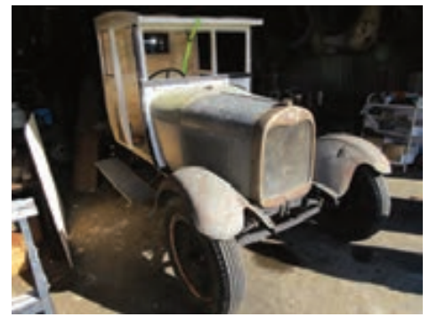
Gisborne: Gavin Bartlett's 1928 Model AA Ford takes shape with the fuel tank, bonnet and radiator now attached to the newly-constructed cab.
