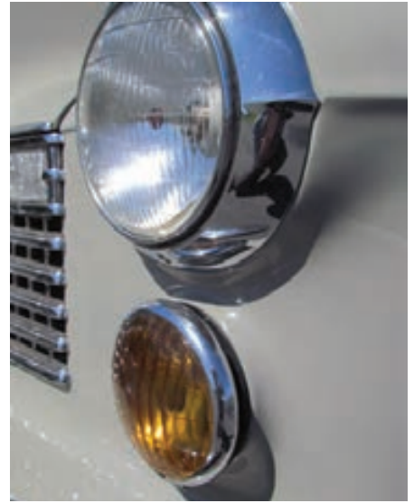
Recessed fog lights are aimed and then locked in position.
