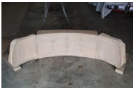
Horowhenua: Moulds to manufacture the MGA 3 piece screen.
