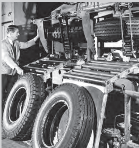
The two truck tyres on the floor have been discharged from a 55-inch McNeil Bag-o-Matic press. Another two are held in the post-inflator, where they are inflated while they cool, so that they will keep their shape; they are held for the time it take for the next pair of tyres to cure; around half an hour. Photographer: National Publicity Studios, Photo uhcl.recollect.co.nz
