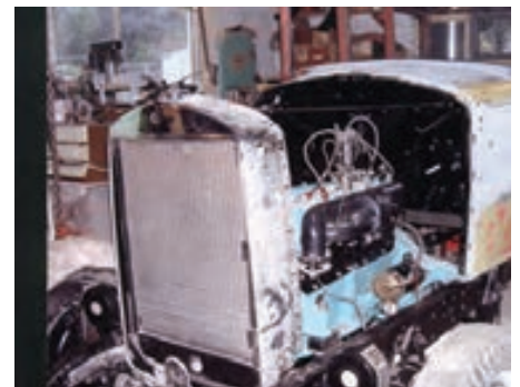
Undercoated body and radiator in position on chassis.
