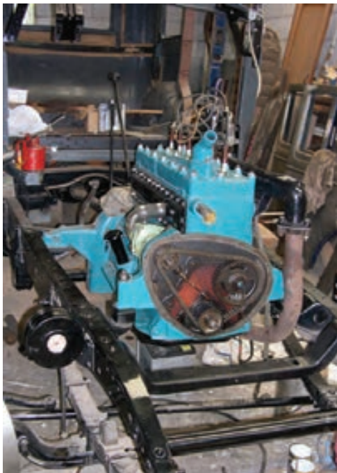
Completed engine mounted in restored chassis.
