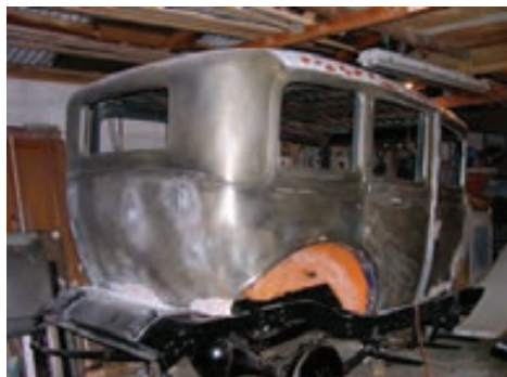
Body stripped back to bare steel, sitting temporarily in position on chassis.
