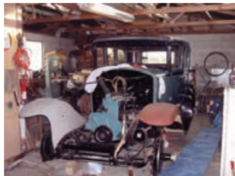
Finish coated body in place on chassis with front mudguards temporarily in place.
