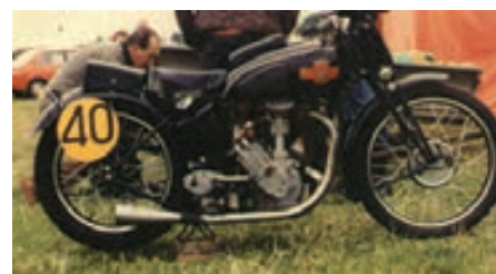
Details on back of photo: 1939 Excelsior Manxman special. Very rare model, believed to be one of 5 by c1950. 500cc, bronze cylinder head, Amal TT carb, Albion gearbox, Girling brakes. NZ owners Marty Rush (new), Jim Oed, Mick Holland. Sold to UK buyer in 2002?
