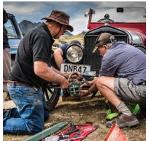
Model T lost a bolt in sump, lost oil pressure and ended up under tow.
