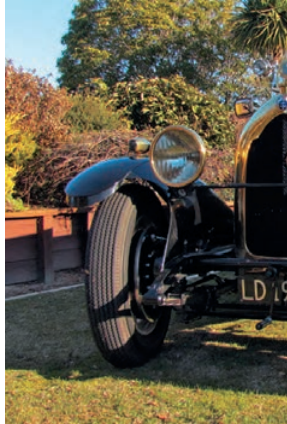
Bentley and Lorraine radiator profiles are not unlike. All bright ware is polished brass – nickel was an option until becoming standard in 1925.
