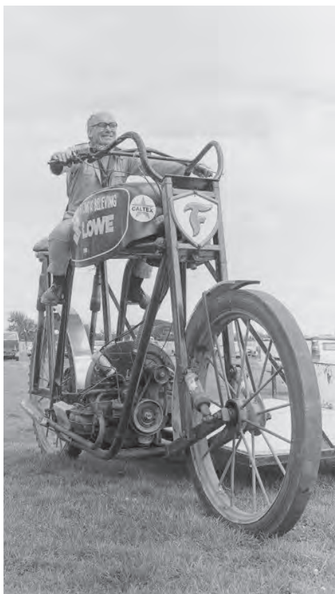
Manawatu: Don Lowe seated on his unique home-made motorbike. The bike stands 2.2 metres high and is powered by a Volkswagen motor. Copyright PAColl - 7327 - 2. Photo originally taken by Stuart Ramson 18 March 1985 ( Evening Post photographer). Historical notes; Don Lowe was the owner of the Bunnythorpe garage at this time. He built his motorbike in two months in 1981 from old farm appliances.
