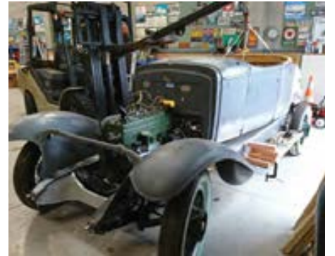
▲ ▼ Auckland: Coming together - Peter Wood's Marquette body being put on the chassis.
