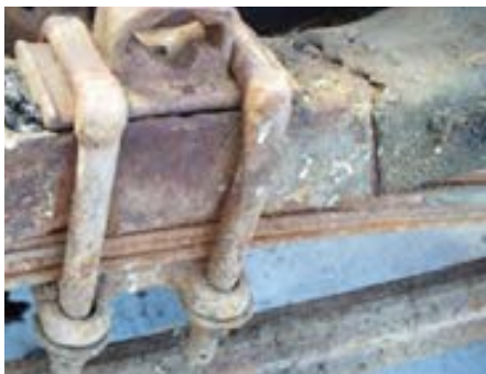
▲ As can be seen from the above photos the bare skeleton is revealed to show a weakened state, especially in the front cross member which had seen an attempt at repair. This was replaced by another cross member.
