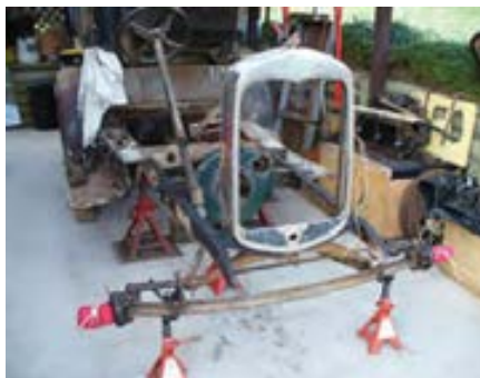
▲ As can be seen from the above photos the bare skeleton is revealed to show a weakened state, especially in the front cross member which had seen an attempt at repair. This was replaced by another cross member.
