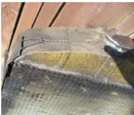
▼ The radiator posed a problem as wire had been used to hold part of it together, a practice that was not confined to just the radiator. This wiring caused the demise of the radiator and a new one had to be sourced
