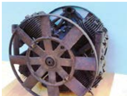
Wellington: Ford's X Engine that never quite worked properly.
