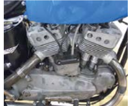
▲ Alf Groves' modifications - the additional magneto and drilled cylinder heads.
