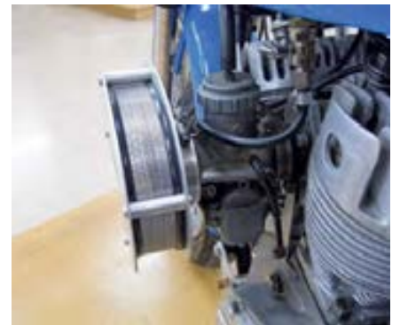
▲ Mikuni carburettor fitted for ease of use.
