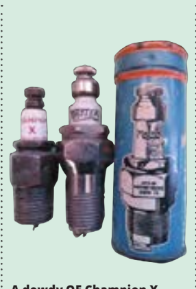
A dowdy OE Champion X is overwhelmed by the Master, Hartford Machine Screw Co's upmarket Ford model sporting nickel plate over polished steel and impressive packaging. Perhaps this version was aimed more at the whole F.O.R.M.S. market.
