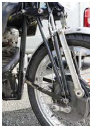
▲ The brake is internal twin leading shoe. The girder have needle rollers on all four pins.
