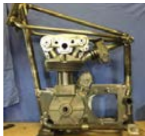
▼ Road frame modified to replicate late works semi-duplex frame.
