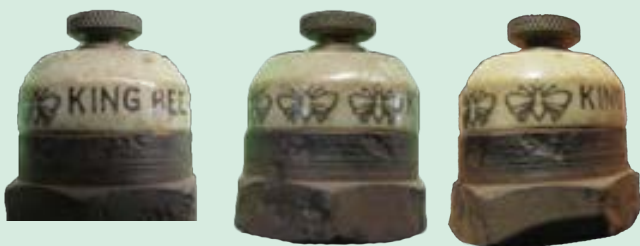
Three little bees decorate this unusual King Bee plug. The outer porcelain is for branding and protection of the inner porcelain that does all the work.
