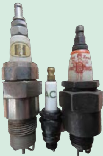
The tiny 10mm plug used by Cadillac and others is dwarfed by Red Head's Big Boy and the nickel-plated Hercules, its logo transfer as the porcelain is not glazed.
