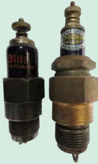
Blitz (Boston, USA) was one of the very few to fire a readable logo on its dark blue porcelains. Benford's Monarch used a paper label on the Blue Adamant porcelain of their Golden Giant model, which was kissed with 24ct gold, some of which remains - eye candy indeed. The Golden Giant was also made with white porcelain.
