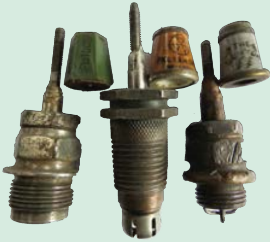
Splitdorf, Hills AAA and The Benton are examples of laterally-wound mica insulators protected by porcelains whose colours, shapes and logos add visual appeal. It can be seen the Benton mica is contaminated with oil.
