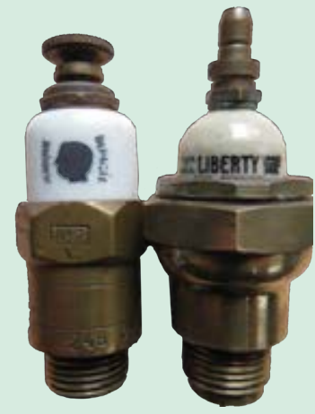
Two examples of all-brass plugs. The needle point of the Liberty (US) plug is designed to release oil drips more readily. Oleo used this head silhouette as their marque déposée (registered trade mark).
