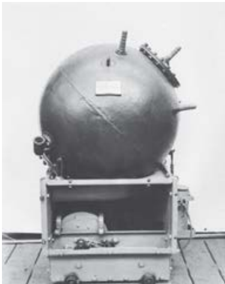
▲ An HZ Mk II mine and a Mk VIII mine sinker. W.R.M. Motors Ltd. made some 50,000 of the latter during the First World War.
