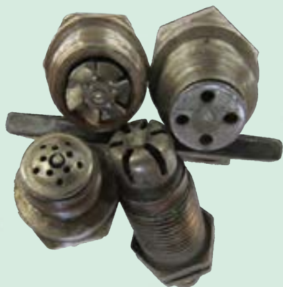
▲ A very large number of brands targeted the electrodes to have a point of difference. Here are four examples of what seemed like a good idea at the time. Clockwise from top left: Fan Flame, Pep, Hills 3-A and McQuaire.
