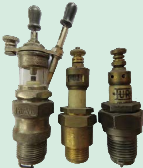
▲ The Rentz "Lighthouse" (US) is the most dramatic of all the spark plugs with built-in intensifiers. The spring-loaded centre electrode can be set to eliminate the gap, but why would you? The side earth bar is used for testing. Composed of 25 pieces this was the most complicated and expensive plug ever made. Action at the adjustable intensifier gap of the brass FZG plug (Germany) can be observed through its little bay window. The Duro (US) intensifier, visible through the small holes, is not shielded from fuel vapour and that design was quite common, surely asking for excitement.
