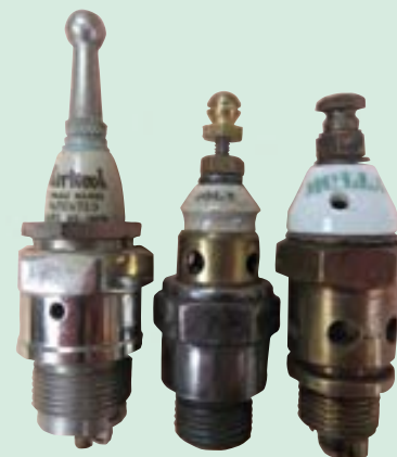
▲ Air-cooled plugs were used mainly in aircraft and motorcycles. The Airkool (US) porcelain is drilled in the back. Molla and Joly ("Jo-Lee") are French plugs; some 5 million Joly plugs were required for WW1 aircraft, many of them produced in the USA by Lyons Ignition Co.
