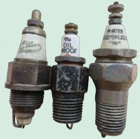
▲ Ezekleen, The Oil Proof and Porter Keepsklean are just three of many plug brand names that referenced the ongoing fight with fouling. It was Ezekleen's exposed porcelain that made it easy to clean. Odd spelling was another common sales ploy.
