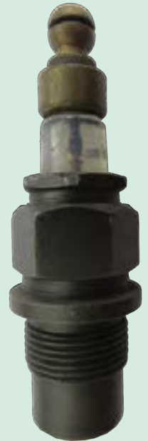
▲ A number of manufacturers produced a plug that provided a view of the explosion. A misfiring plug was obvious while the colour of combustion provided a useful diagnostic tool. This Beacon Lite (US) with its "Visible Flash" Opalite core dates from 1922.
