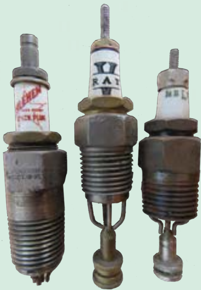
▲ Bethlehem, V-Ray and HeLfi (all US) offered the motorist improved odds with four earth electrodes (the meaning of Five Point on the Bethlehem plug). V-Ray and HeLfi are equipped with a drilled terminal nut that has a serrated bevel, shown here in position to clean and true the four earth electrodes.
