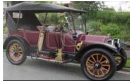
1914 BUICK MODEL B - 25X TOURING CAR. 165 ci engine, 28 hp capacity, 105" wheelbase. One of the 1544 built for export. Imported by NZ Automobiles Ltd, first sold by Buick sub-agent, W O Callaghan Motors, Hawera. Very good restored condition. Ph Neil 03 434 9470, neil.nonie@xtra.co.nz MEM NTH OTAGO
