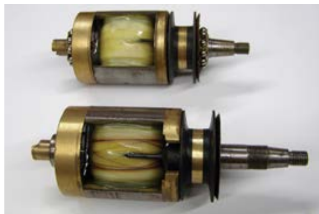
▲ Lucas rotating coil armatures - lower one is from a Magdyno
