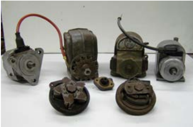
▲ (L to R) Magnetos - BTH Flange mounted, Lucas SR1, early BTH twin. Lucas facecam. (Front row LtoR) Advance and Retard units - BTH and Lucas.
