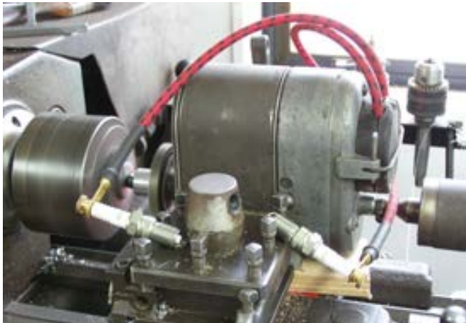
▲ Testing a Splitdorf on the lathe
