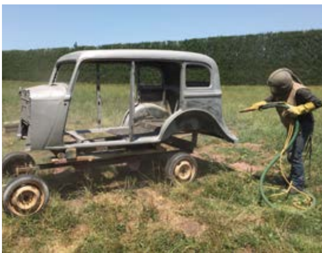
The mobile grit blaster at work.
