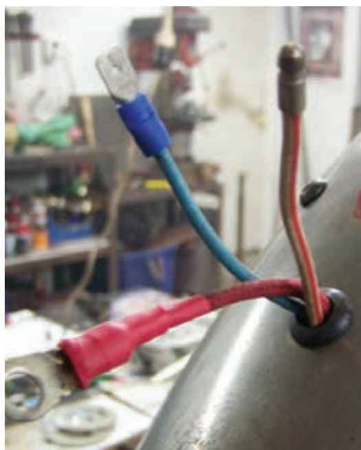
▲ Always use a grommet when running wires through a panel or mudguard
