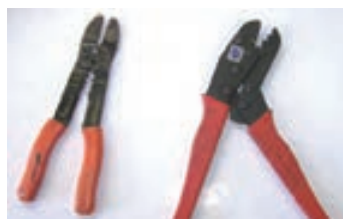
Crimp pliers - inadequate DIY pliers on the left and professional pliers on the right.
