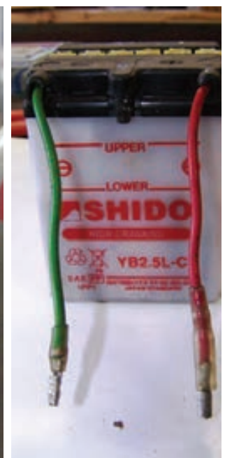
▲ Motorcycle battery with Japanese standard male and female bullet connectors
