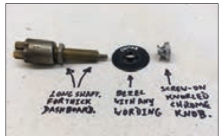
TWO LUCAS P87 PULL-PUSH SWITCHES wanted as in photo. They have a long shaft to go through a thick dashboard (engraved wording on bezels is immaterial) and have knurled chromed screw-on knobs. Please contact Monty 02 -022 61295 MEM CANTERBURY
