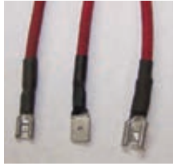
Disguised crimp connectors
