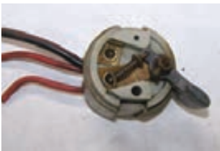
▲ Motorcycle dip switch mechanism
