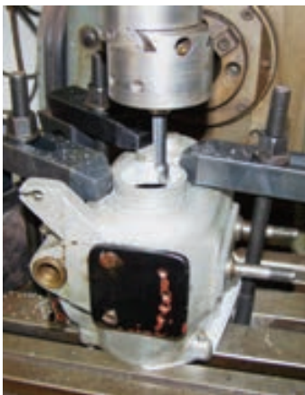
Reboring the gearbox casing.
