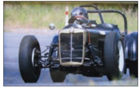
MGV . Built and campaigned by Trevor Crowe from the early '60s. Modified 284ci 99A V8 Mercury. Lincoln high ratio gears, Mercury 3.54 diff, certified roll bar, on racing Dunlops. Huge history. Performing very well and eligible for many events. $35,000. Ph 03 312 3112 MEM CANTERBURY
