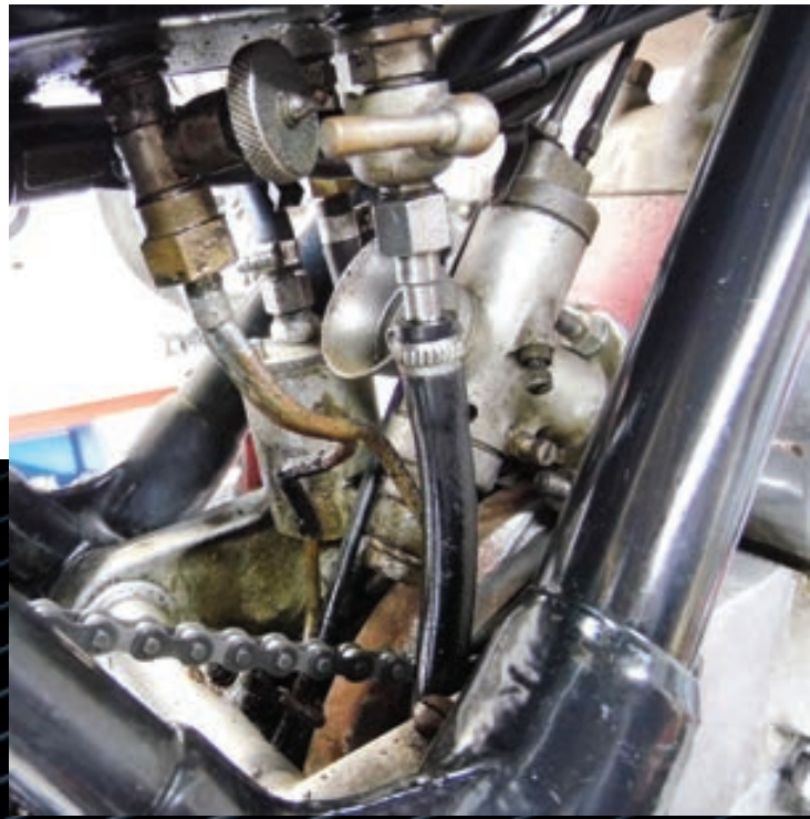
The engine room - note the unique to Scott carburettor.
