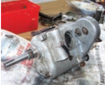
Gearbox note extended output shaft.
